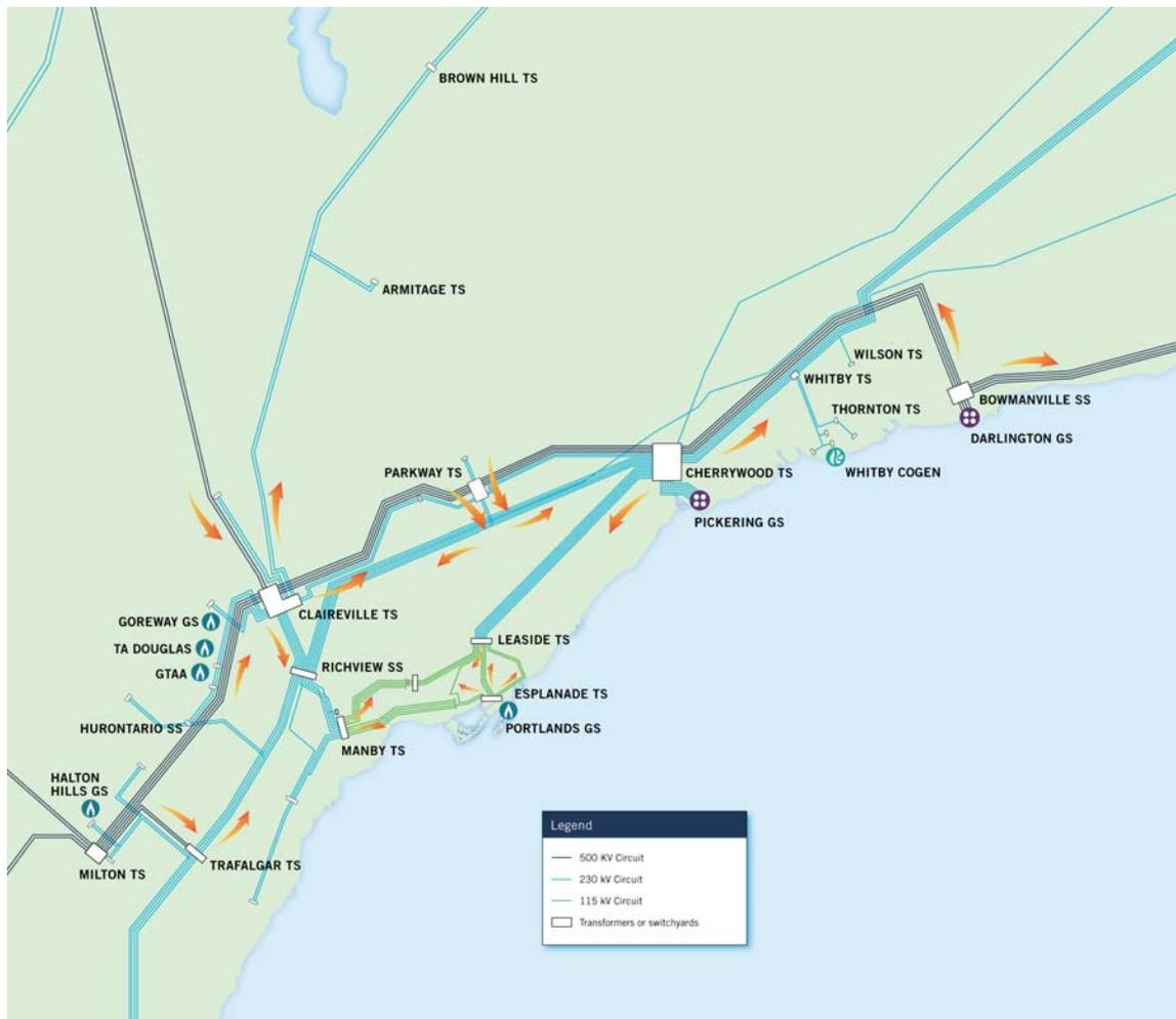
The reliable supply of demand in the GTA under extreme weather conditions forecasted for the Outlook period requires a minimum number of autotransformers at Trafalgar, Claireville, Parkway and Cherrywood and Pickering units in service at rated capabilities. For summer 2009, all autotransformers and Pickering units are expected to be in service. The projected loadings on
