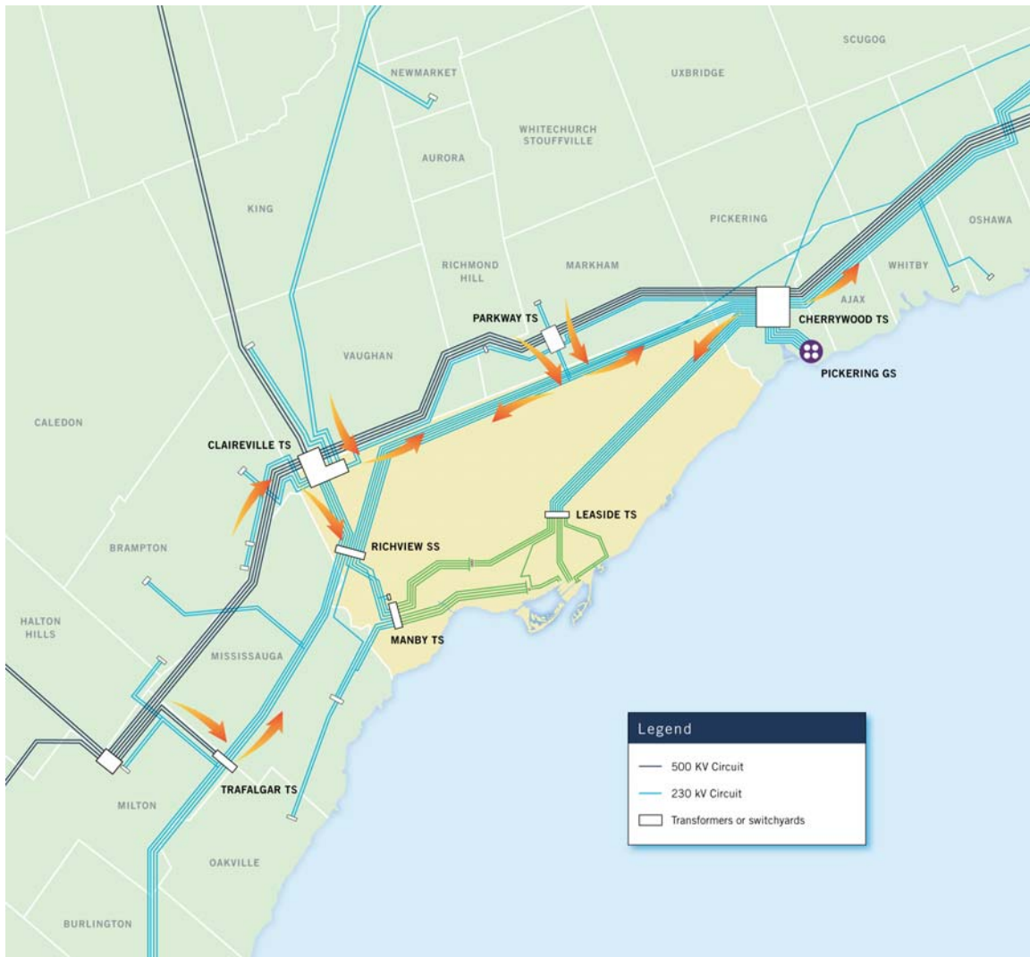
Figure 6.1 Greater Toronto Area Electricity System
