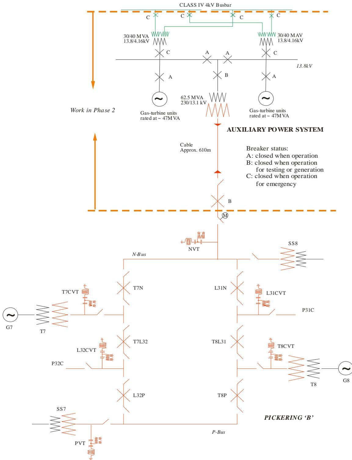
**Figure 1. Proposed Connection of Pickering APS Project**
