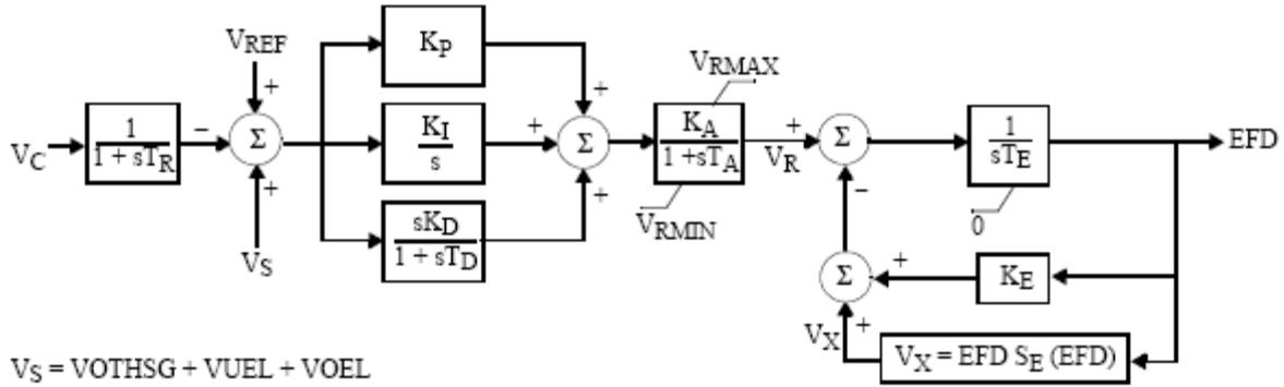
**Figure 2. Excitation System Block Diagram**
