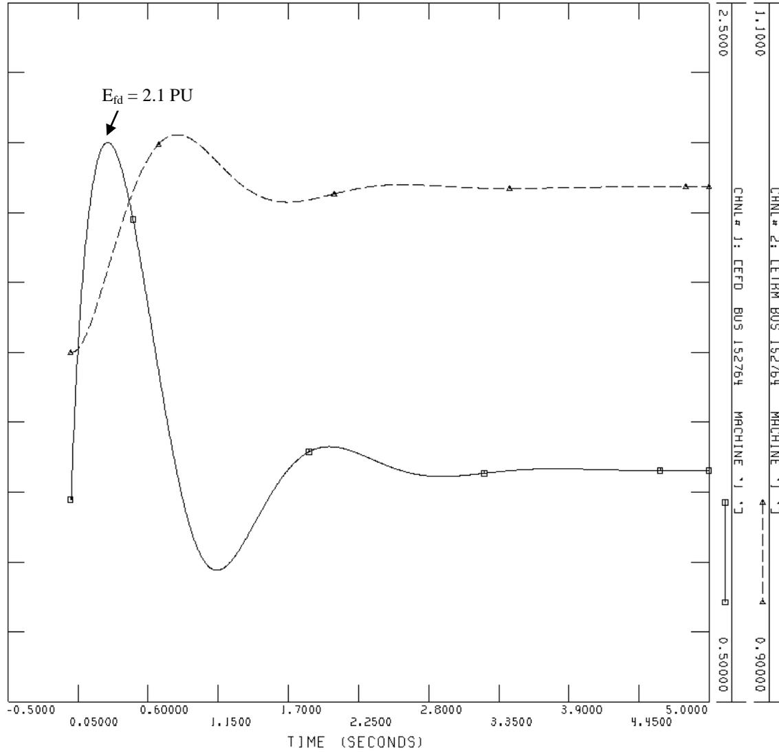
**Figure 3: Positive ceiling voltage response time**
