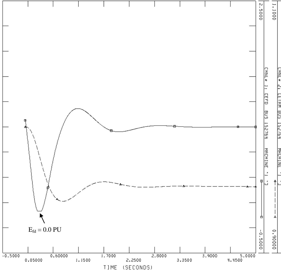
**Figure 4: Negative ceiling voltage response time**
